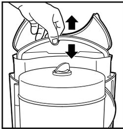
reservoir cover and raise the removable reservoir handle. Lift out the removable reservoir and fill with water to desired level.
